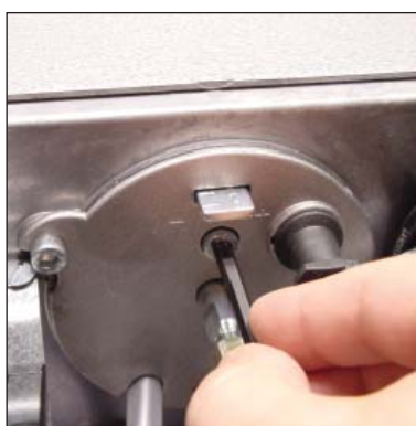
fig. 15 : Combustion head adjuster screw
